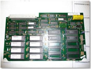
Prepare a 66cm long (from memory, I may be wrong) twin wire with a 2-pin 100mil-pich connector end. Prepare the other end with 2-mm long tinned tips. Unscrew the A11 front panel board and solder the two wires to the pictured solder pads of the flat wire connector. Put the panel back and route the wires as displayed. Attach the connector to the module and sit the A18 board back in place.
