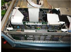
Remove U440 from its socket. Check its orientation is correct like in the picture here.
